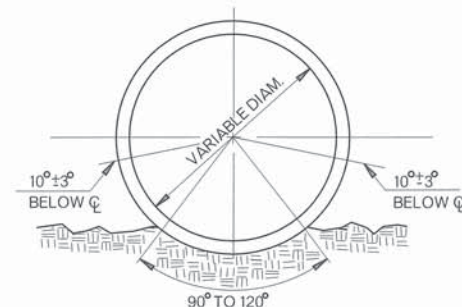
POLYVINYL (PVC) PIPE UNDERDRAIN
